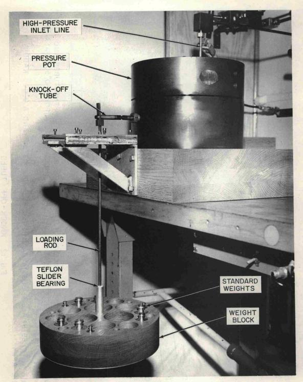
WEIGHT BLOCK CAN BE HELD STATIONARY OR BE ELEVATED IS INCHES AND RELEASED
